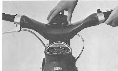
CUSTOM FRONT SECTION GROUP includes detachable handle bar, chrome fender and adjustable headlight. (This modification is necessary for stowing the Suitcase Cycle in the Fiberglass Suitcases.)
