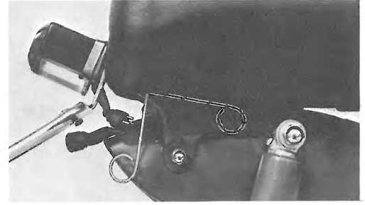
S & K Seat Lock secures seat until it is desired to quickly remove it.
