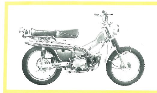
HONDA CT90 — automatic clutc 4 street gears and 4 trail gear swivel handle bars, spark arrests runs on aviation fuel.
