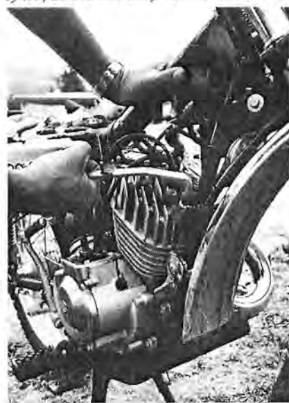
Suzuki disassembles into units that will fit into any four-place plane. Front and rear frame pieces unbolt (below) with wrench that comes with cycle, and is the only tool needed.
