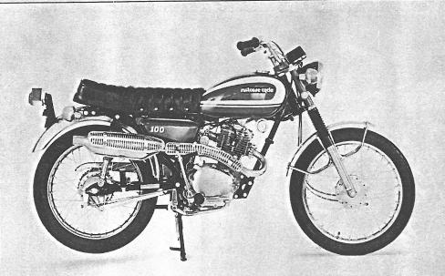
**SUITCASE HONCHO** is designed primarily for street riding but can climb a 35° incline. It carries two people comfortably and is an excellent general-purpose motorcycle. Features a 2-cycle, rotary-valve engine with automatic oil injection.
