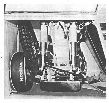
All components of the Suitcase Cycle can be carried in the baggage compartment except for the front wheel which must be stowed on the cabin floor forward of the rear seat:
