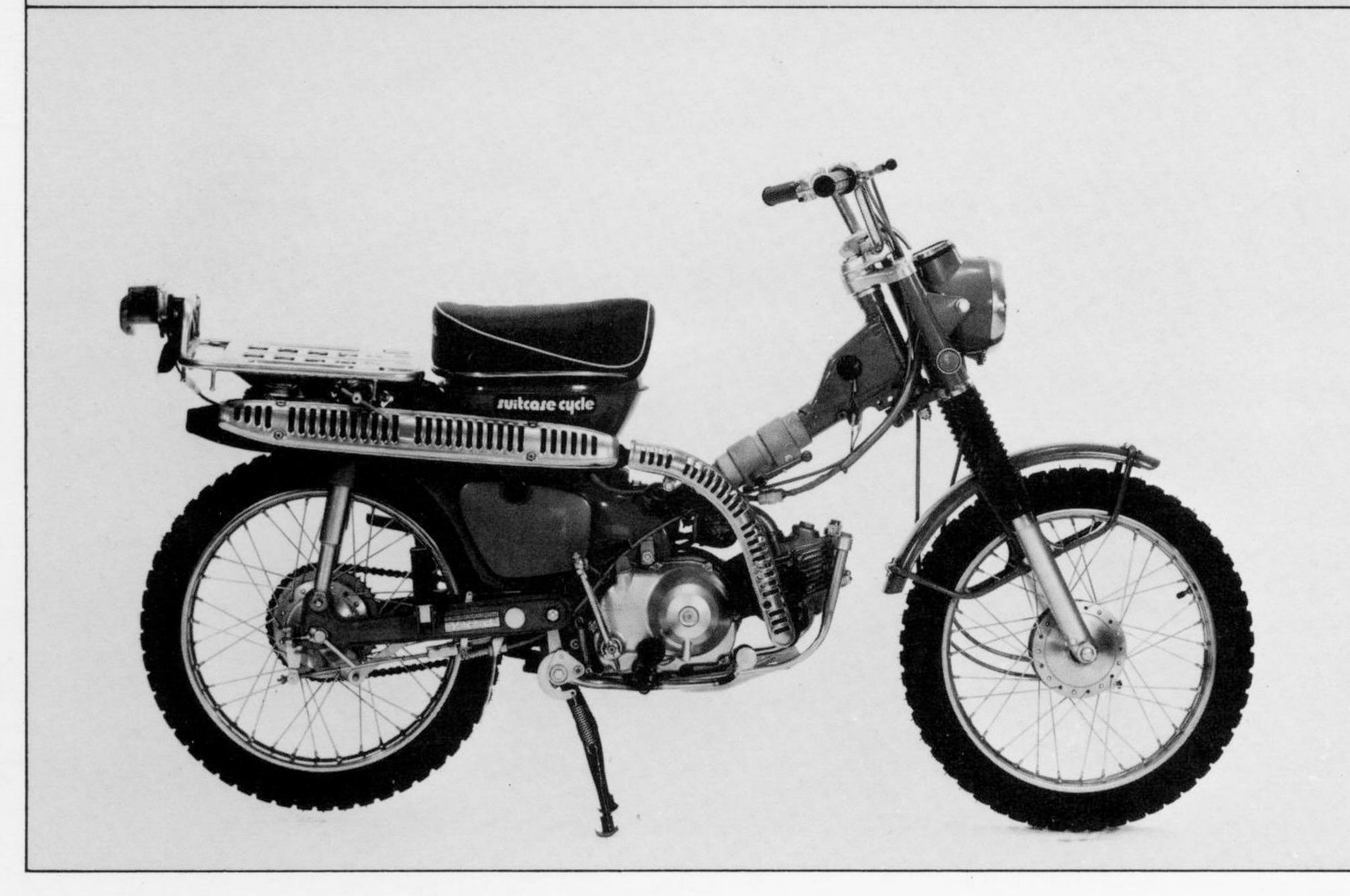
**SUITCASE TRAIL 90** is uniquely suited for trail riding and has swivel handlebars to facilitate stowing. Its step-through frame and automatic clutch make it ideal for women. Features a 4-cycle engine.
